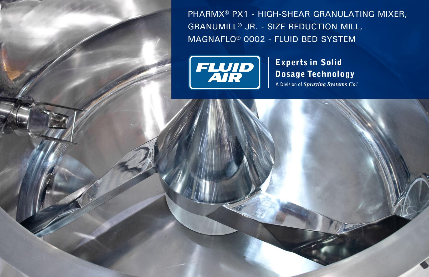
PHARMX® PX1 - HIGH-SHEAR GRANULATING MIXER,
